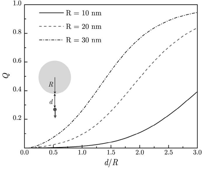
FIG. 1. Fluorescence quantum efficiency for a QE near spherical Au NP is shown vs. QE-NP distance for several NP sizes.
