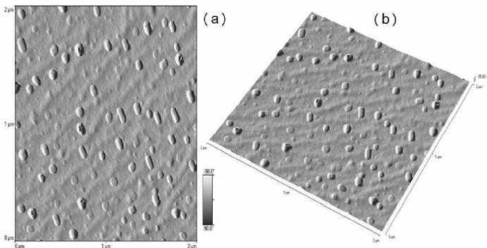
**Figure 2.** AFM images of InAsSbP type-II ellipsoidal QDs in plane – (a) and oblique – (b) view.
