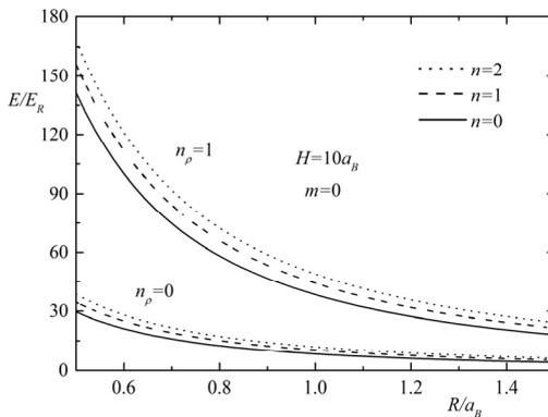
**Fig. 1. The dependence of the energy levels of the electron from the base radius of CQD for the fixed value of the height**
