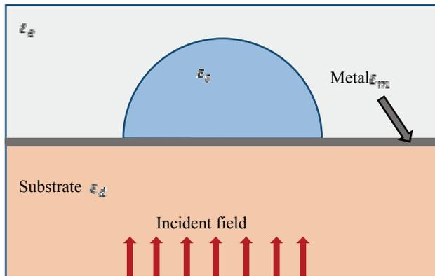
**Fig. 1. Cross section of semicylindrical microresonator.**
