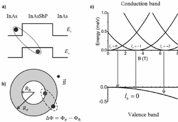
**Figure 1.** Schematic band structure of type-II QD – (a). The sketch of an electron-hole pair in type-II quantum dot – (b). The system energy spectra in magnetic field – (c).
