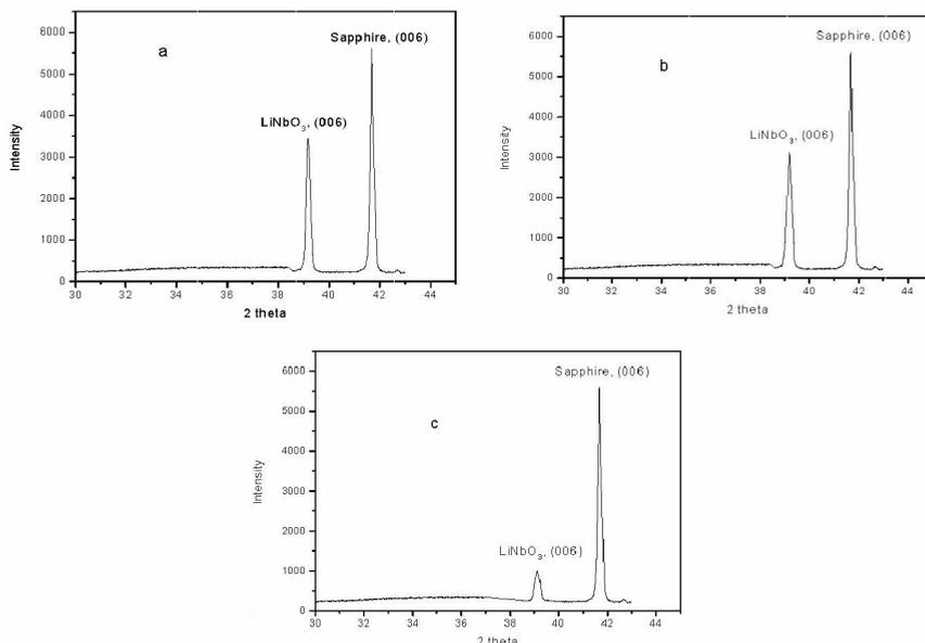
**Fig. 3. X-ray diffraction patterns of thin films. with different thickness**
