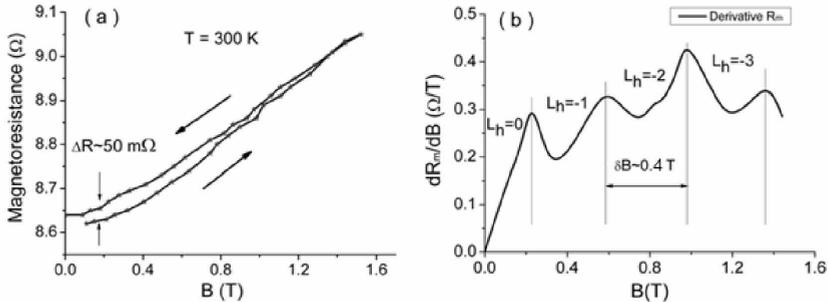
Figure 3. Type-II QDs structure's resistance versus magnetic field at room temperature – (a) and its derivative – (b).
