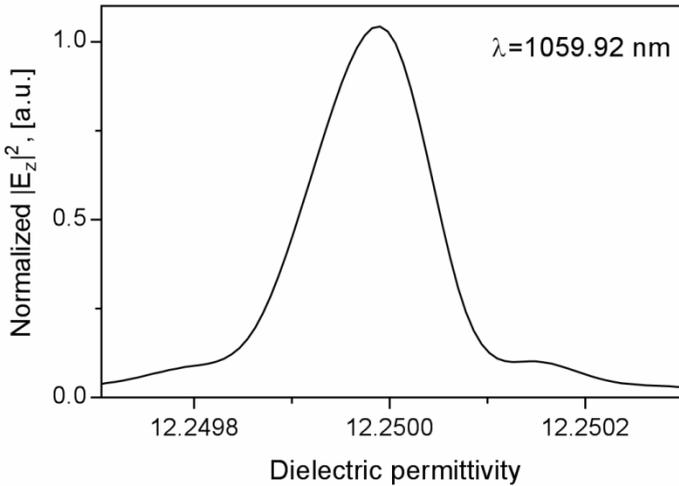
**Fig. 3. Dependence of the square of electric field amplitude on the dielectric constant of a half-cylinder for resonant wavelength  $\lambda = 1059.92$  nm.**
