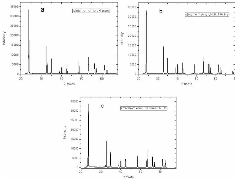
**Fig. 1. X-ray diffraction patterns of synthesized  $\text{LiNbO}_3$  powders of stoichiometric composition doped with different concentration (a-0mol%, b-0.1mol%, c-1.0mol%) of  $\text{Ho}^{3+}$  ions.**
