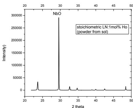
**Fig. 2. X-ray diffraction pattern of fired ready-made Ho-doped lithium niobate alkoxide.**
