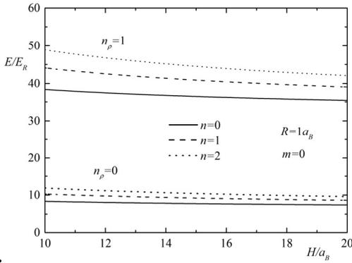
**Fig. 2. The dependence of the energy levels of the electron from the height of CQD for the fixed value of the base radius.**
