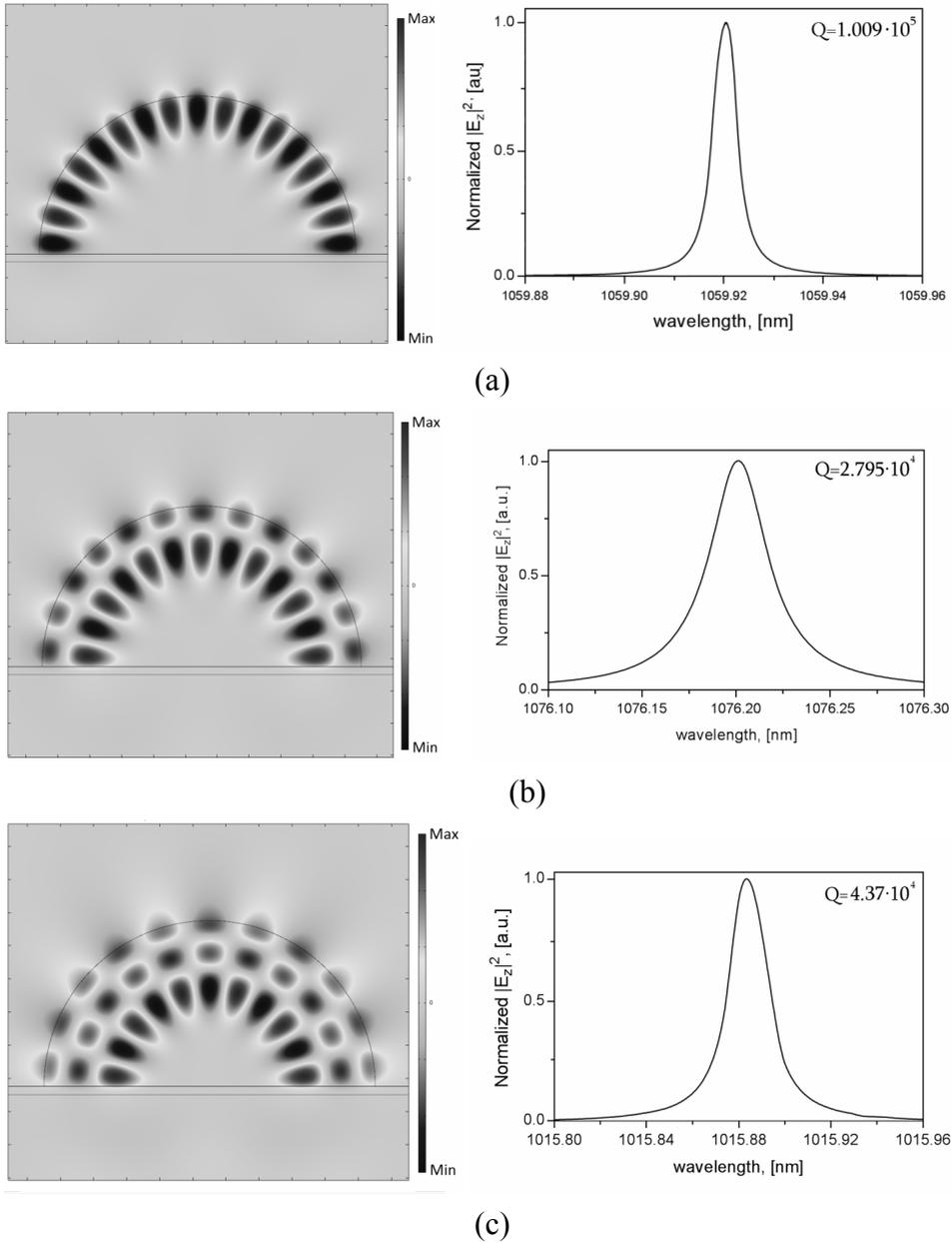
**Fig. 2. The square of electric field amplitudes distributions in microresonator and resonance curves for different wavelength regions.**
